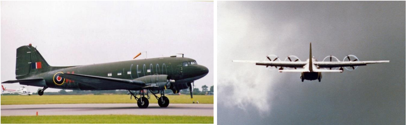
Above: Propeller tip vortices on a DC-3 and C-130 Hercules taking off
