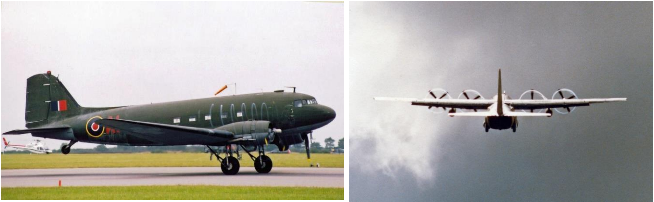
Above: Propeller tip vortices on a DC-3 and C-130 Hercules taking off
